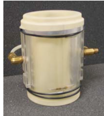
Figure 3. Test Cell Preparation. The following 3 pages, 9 steps, show the basic method used to prepare a triaxial experiment specimen.
