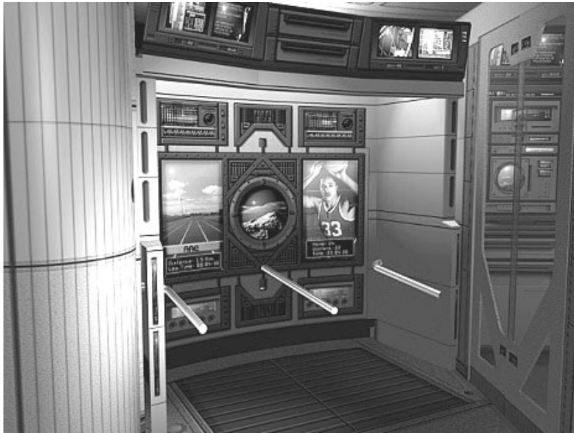
Figure 3-23 The crew exercise facility component of the countermeasures system designed to inhibit crew degradation from exposure to reduced gravity environments.
